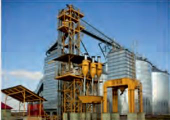
Grain-cleaning and drying equipment as well as storage tanks
